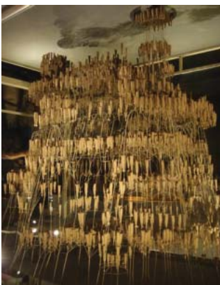
(L)Gaudi Hanging Chain Model (inverted) (R) Reiser + Umemoto Catenary Experiments
